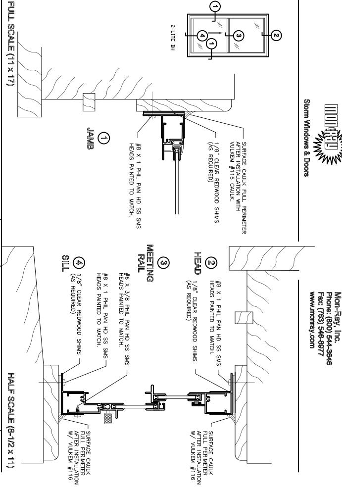
MON-RAY MODEL 500 SERIES - F-CHANNEL ON WOOD DOUBLE HUNG WITH 1855 F-CHANNEL SHOWN
